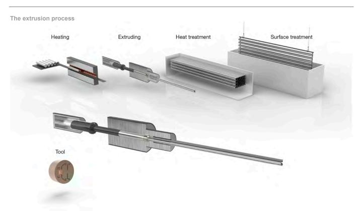
The ingots are preheated, extruded through a die and hardened before surface treatment.
