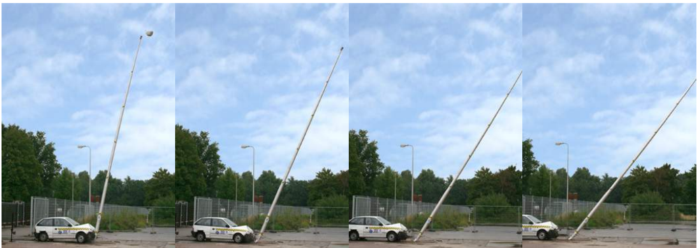
Frontal impact – 100-LE-C crash test
