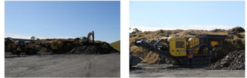
Crushing of 3,000T of refractory bricks for ABF2 ramp construction
