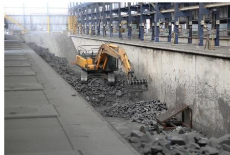
Sorting 1 st Cut SPL in ABF2N using a 200mm sieve bucket
