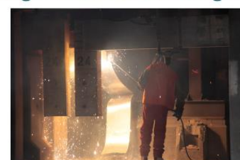
Lancing of anode flexes in Line 1.
