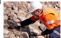
Validation sampling of concrete from the Casthouse (20/7/18). Results show that the concrete is suitable for backfilling.
