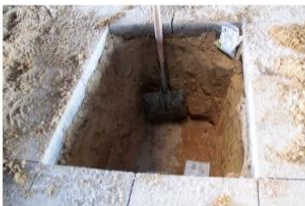
Test pits dug down to natural clays and soil samples taken at progressive intervals
