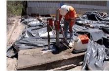
Coring of PCB-impacted concrete slabs and sectioning for concentration profile analysis (20/11/18)
