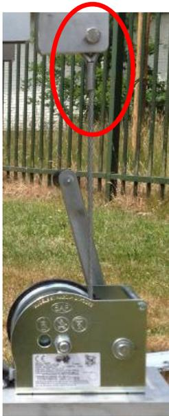
**Note:** Check all connections are secured and make sure that the cable is secured. Ensure the cable is tightened prior to loosening captive bolts. This to check if all is secured! Then move on to the “lowering and raising of the hinged column”, *Section 7*.
