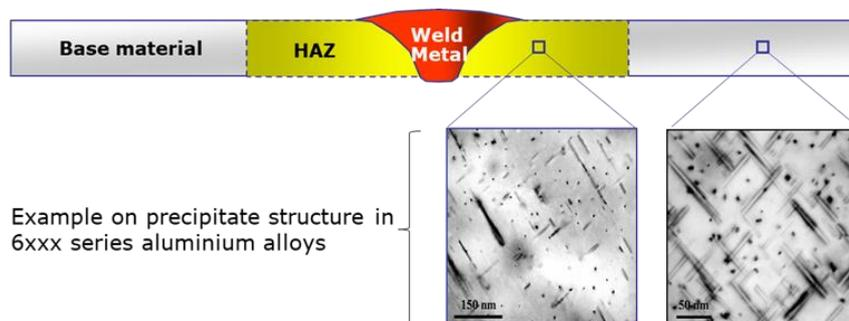
> Figure 3-10 Cross-section of welded joint
