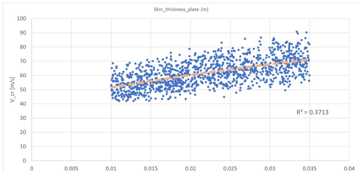
> *Figure 4-6 Critical wind speed with respect to the skin thickness of the top and bottom plate*
