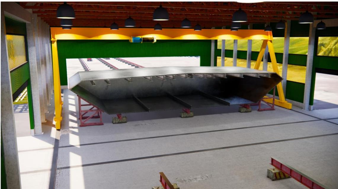
6. Skid the first sub-section 12m out of the workshop to prepare for the next sub-section
