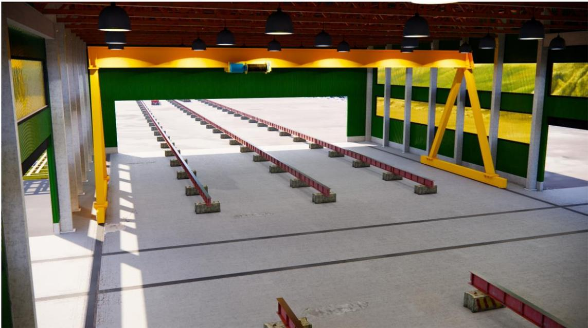
2. Start with the bottom deck panel, locate on the skid tracks
