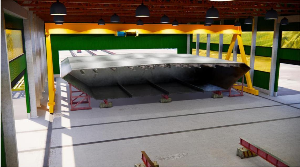
9. Assembly of two 120m-sections in parallel by feeding the panels through the mid-gate of the workshop, the gantry crane can be operated at both workshop ends.
