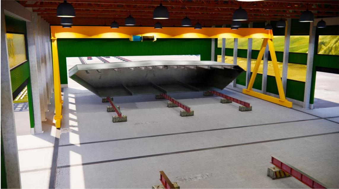
7. Form the next sub-section according to the same sequence as for the first, but also join the parts together with the first sub-section.
