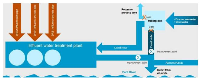
Figure 4.16 Principle of effluent treatment plant at Alunorte
