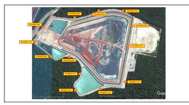
Figure 4.23 Monitoring wells at DRS2
