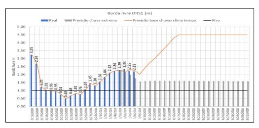
*Figure 4.3: The variations in the freeboard (borda livre) in DRS1 as measured (taken from the Alunorte Plant Operations system - blue is actual, grey is forecast for extreme situation)*
