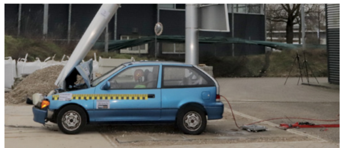
Crash test shows safety of crash-friendly pole
