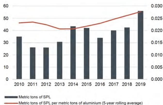
The volumes of spent potlining (SPL) varies with the relining of smelter cells which is normally done every 4-7 years for established smelters. Furthermore, opening new production lines and closing down production lines will give fluctuations in the aluminium production, and - due to the cyclical nature of SPL - a 4.7 years time lag in the SPL volumes. Hence SPL is normalized with aluminium production with a 5-year rolling average as the best estimate of a trend line.
