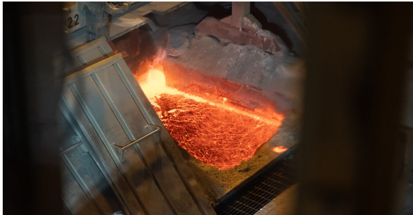
The cryolite bath in an electrolytic cell is maintained at around 960-980°C.
